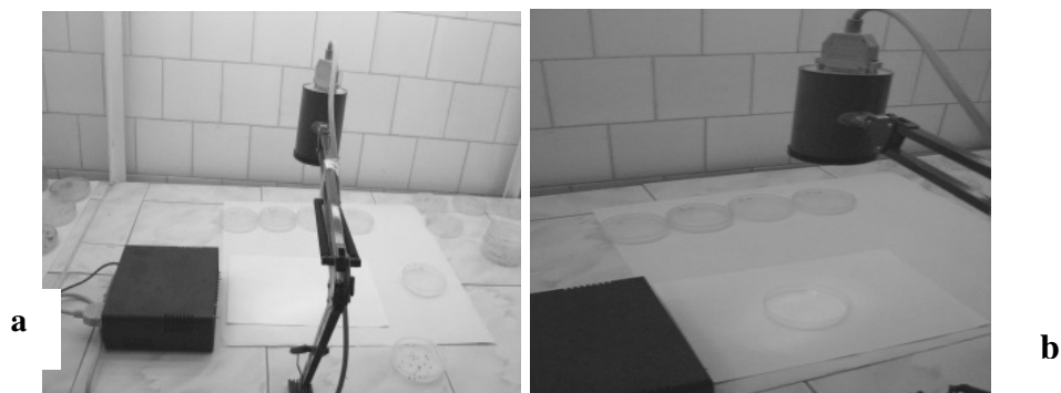
Figure 1. Experimental device unit attachment with diode laser irradiation (a) and seed treatments on Solanum melongena (b)
