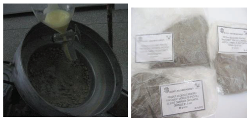
Figure 4. Vegetable oil-based product formulation using a rotating drum granulator
