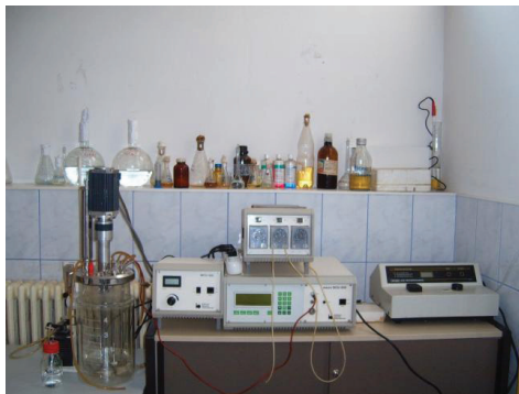
Figure 1. Laboratory plant for biogas production
